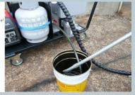
After-use cleaning can be done easily with circulation mechanism using light oil. Use of empty pail enables safe cleaning at a distance from the high temp sections of the machine.
